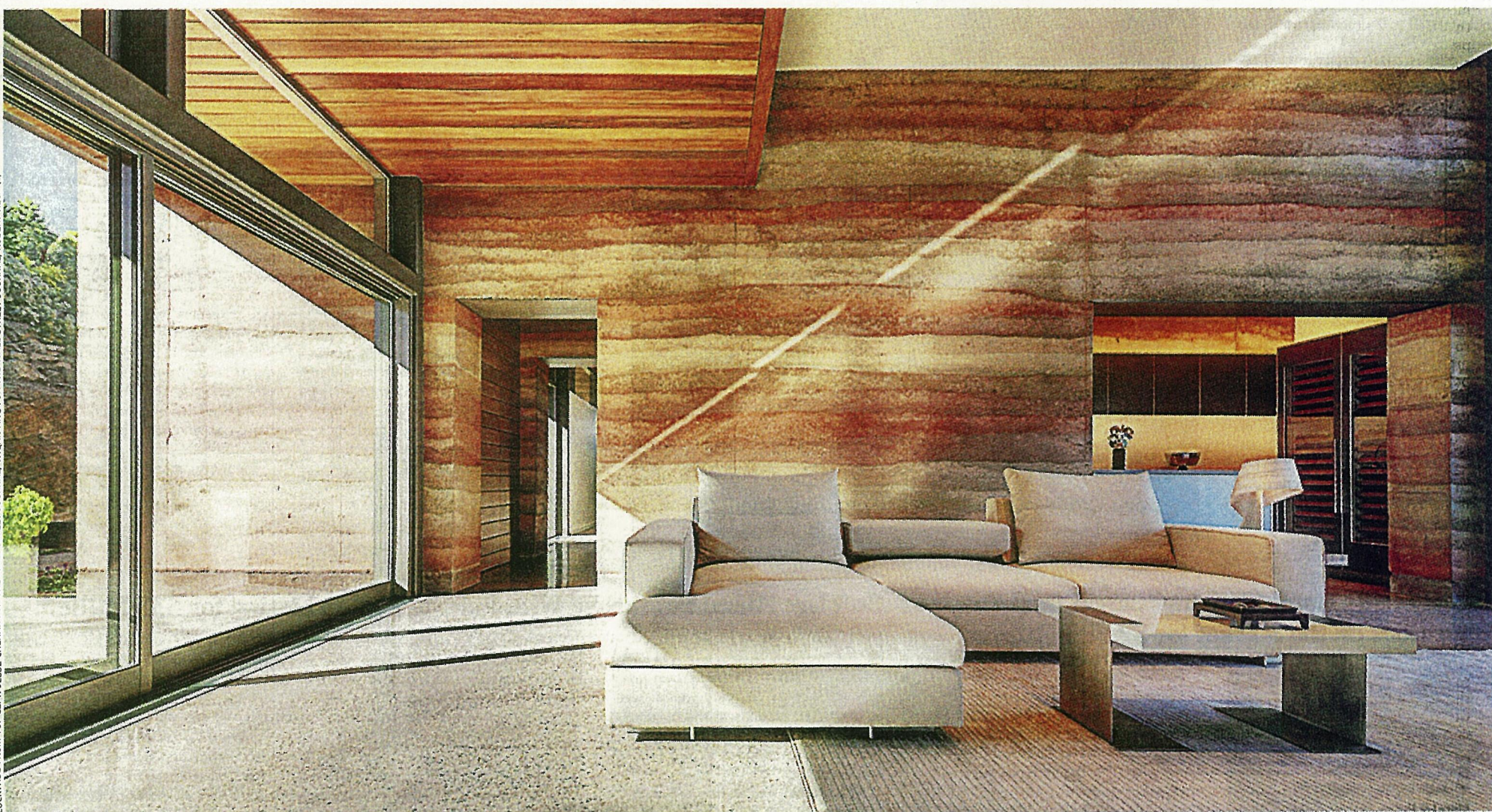
LAYERS OF WARMTH Rick Torcasso's rammed-earth builder used iron-oxide pigments to dye the earthen mixture four different colors, giving the walls a striated pattern. Mr. Torcasso said that the walls of his Santa Fe home are efficient as well as good-looking, noting that over a three-day period when outdoor temperatures hovered in the teens, the heating system in the main living area was in use only 20% of the time.
