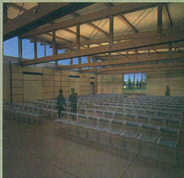
DOWN AND DIRTY Sublette County Library's community room (upper left rendering) will have three walls of rammed earth. The external rendering (upper right) shows the photovoltaic panel. The construction photo displays a close-up of the "sunset effect" of the tinted earth
